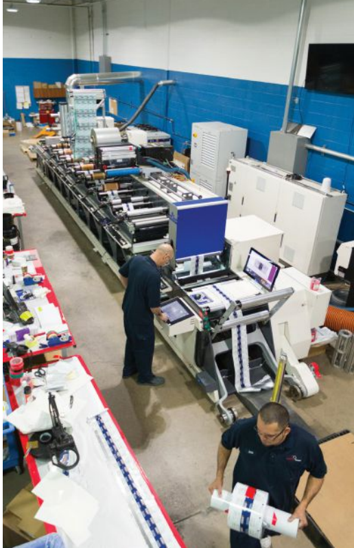
Makeready materials are removed from the 22" Nilpeter press.
